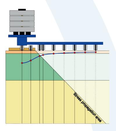
If your add an extra geophone at 100mm from the center of the load, inside the load plate, the additional 100mm geophone improves the accuracy of the deflection bowl trend.
