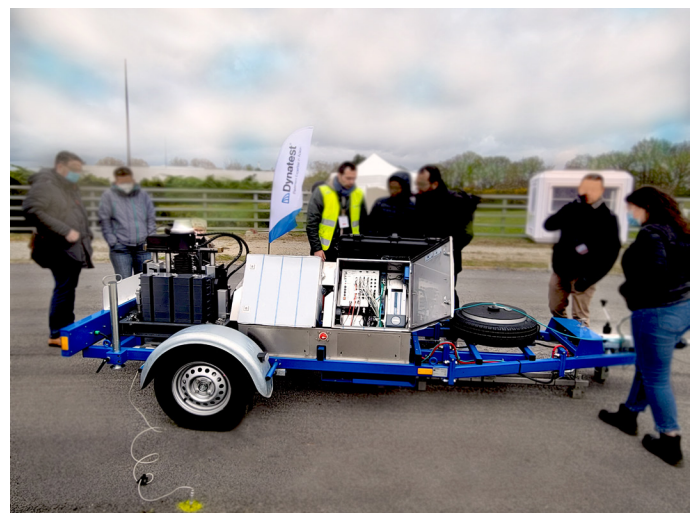
Given the productivity improvements of the FastFWD it is natural to study the possibility of using the device for in-situ Accelerated Pavement Testing (iAPT). Here demonstrated at the APT Conference 2022.
