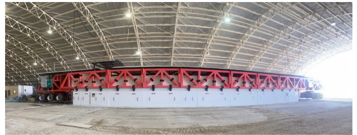
The most widely used mobile device is the Heavy Vehicle Simulator (HVS). This one is the Dynatest Titan 2022.
