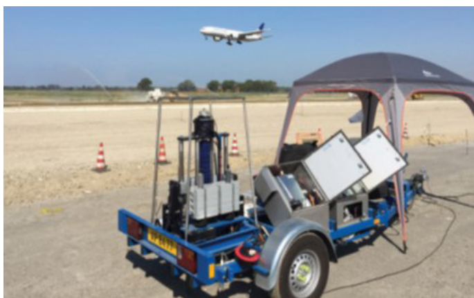
In Accelerated Pavement Testing applications, the FastFWD will be placed in the same spot for as long as the testing demands.
