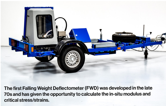
In 2015, the Fast Falling Weight Deflectometer (FastFWD) was introduced speeding up testing procedures and overall productivity reaching a loading rate from 5 to 7.5 times faster than any existing FWD device.
