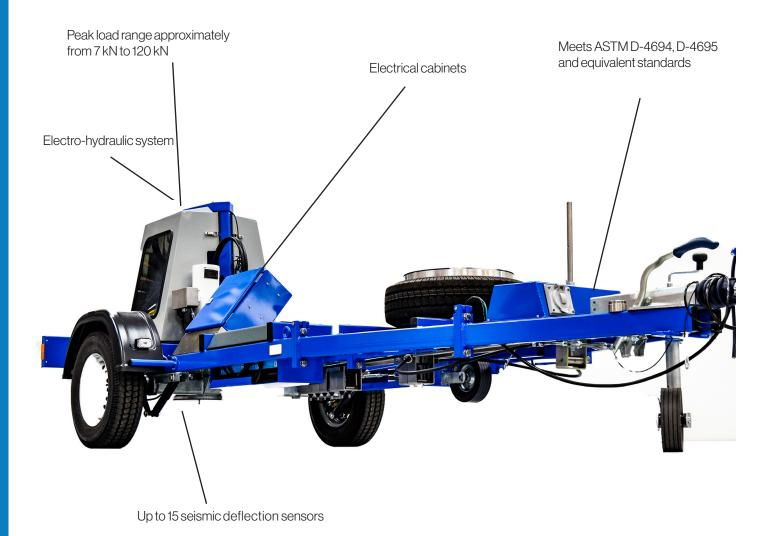
The Falling Weight Deflectometer (FWD) is an integral part of the process for structural evaluation of pavements and for a good reason. The FWD is a non-destructive and fast method to evaluate the structural capacity of pavements for research, design, rehabilitation of the road and for pavement management purposes.
