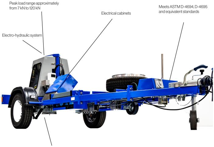
Up to 15 seismic deflection sensors
