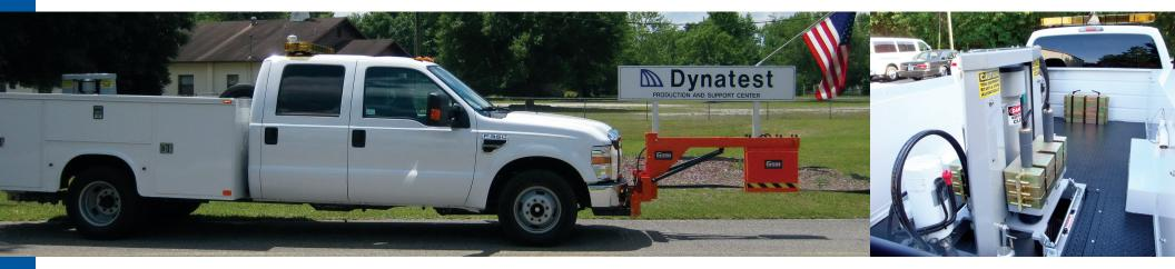
As with all members of the Dynatest Model 8000 and Model 8081 Falling and Heavy Weight Deflectometer product lines (FWD and HWD), the TMD provides fully automated, fast, highly accurate and precise measurements suitable for use with standard analysis and design procedures including especially rigorous mechanistic-empirical analysis of pavement structures such as the proprietary Dynatest ELMOD (Evaluation of Layer Moduli and Overlay Design) program.
