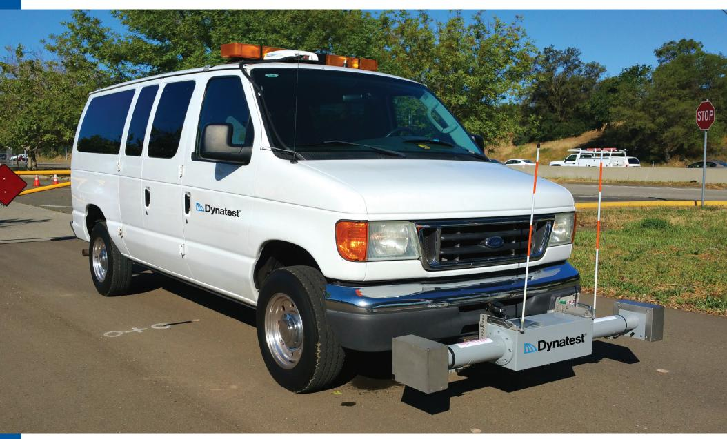
Dynatest portable Road Surface Profiler (RSP) Mark IV is designed to provide advanced, automated, high quality pavement roughness measurements for engineers, construction superintendents, and pavement network managers. The portable RSP Mark IV can be fitted easily to most vehicles.
