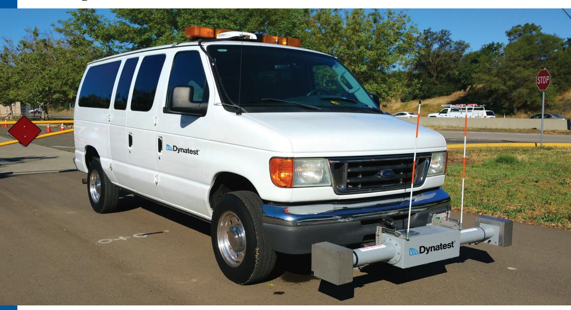
Dynatest portable Road Surface Profiler (RSP) Mark IV is designed to provide advanced, automated, high quality pavement roughness measurements for engineers, construction superintendents, and pavement network managers. The portable RSP Mark IV can be fitted easily to most vehicles.
