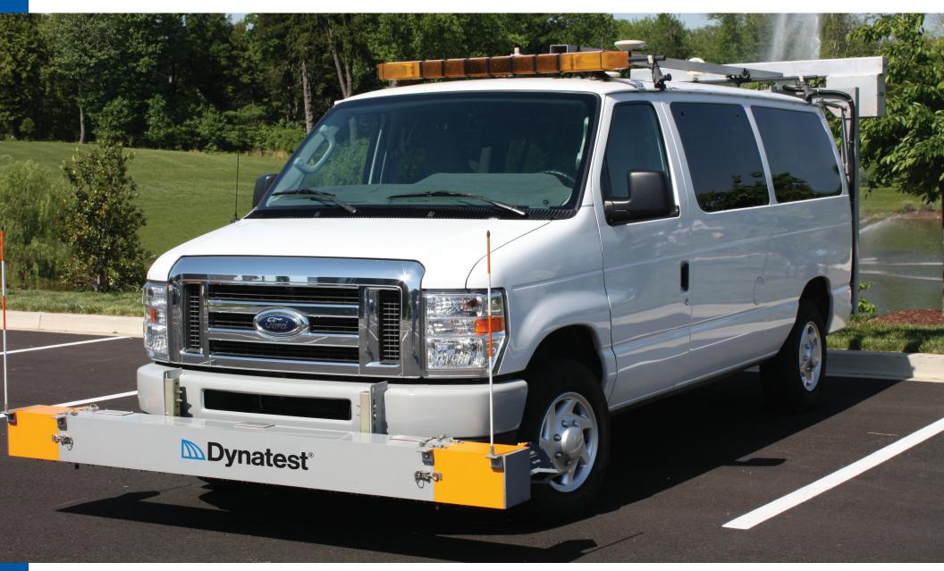
Dynatest Road Surface Profiler (RSP) 5051 Mark III is designed to provide advanced, automated, high quality pavement longitudinal and transverse profile measurements for engineers, construction superintendents, and pavement network managers.
