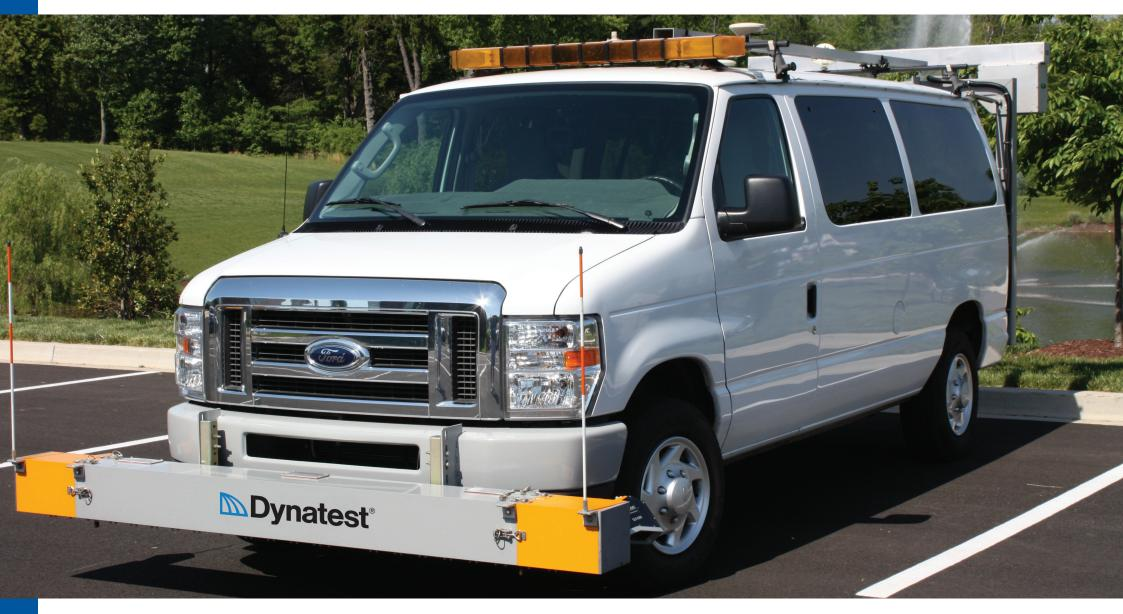
Dynatest Road Surface Profiler (RSP) 5051 Mark III is designed to provide advanced, automated, high quality pavement longitudinal and transverse profile measurements for engineers, construction superintendents, and pavement network managers.
