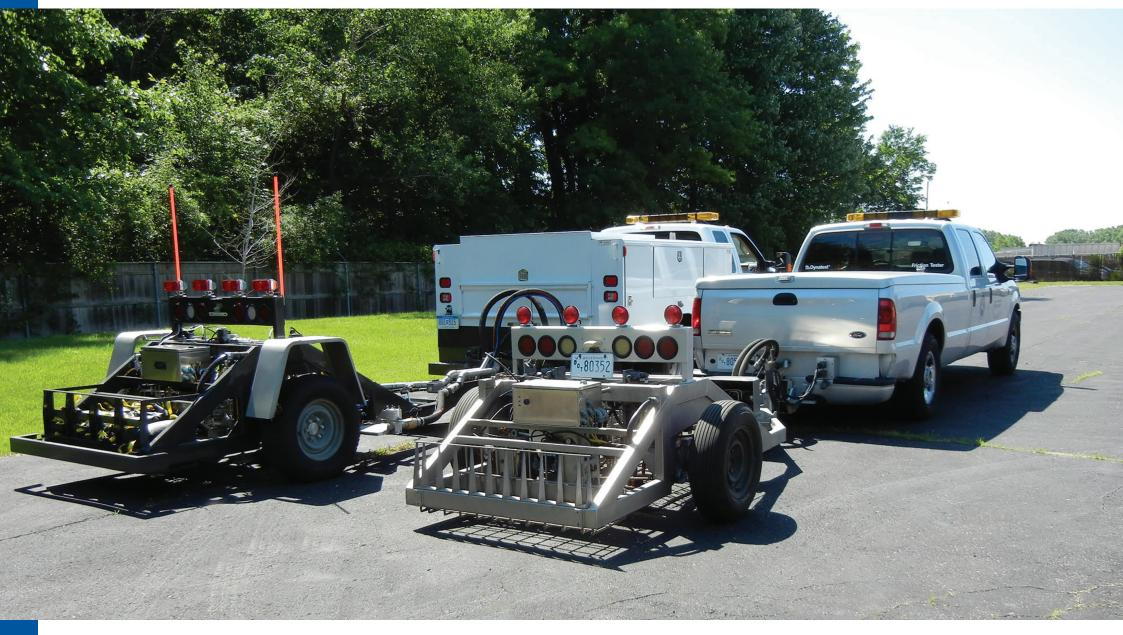
The Dynatest 995 Tire Traction Tester (TTT) measures both the locked wheel (slide) and peak (slip) friction characteristics of tires on dry or wet pavements at speed ranging from 30 to 110 KPH.
