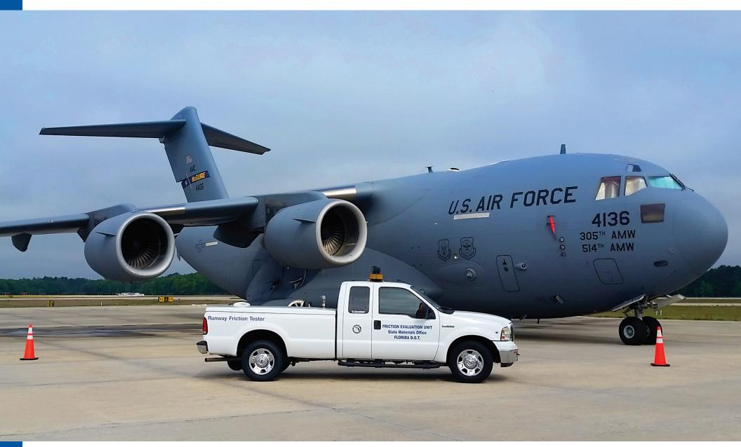
The Dynatest 6875 Runway Friction Tester (RFT) is designed to measure runway friction characteristics for both pavement maintenance and operational purposes. Pavement maintenance to address runway friction concerns may be required due to rubber contamination or weathering of
