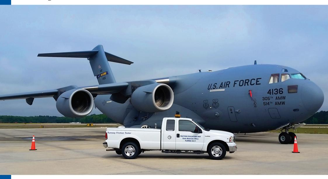
The Dynatest 6875 Runway Friction Tester (RFT) is designed to measure runway friction characteristics for both pavement maintenance and operational purposes. Pavement maintenance to address runway friction concerns may be required due to rubber contamination or weathering of the pavement surface.
