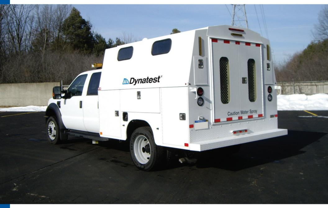
The Dynatest 6875H Highway Friction Tester is designed for maintenance testing to evaluate changes in highway pavement friction characteristics due to weathering, polishing, aging, and contaminants.
