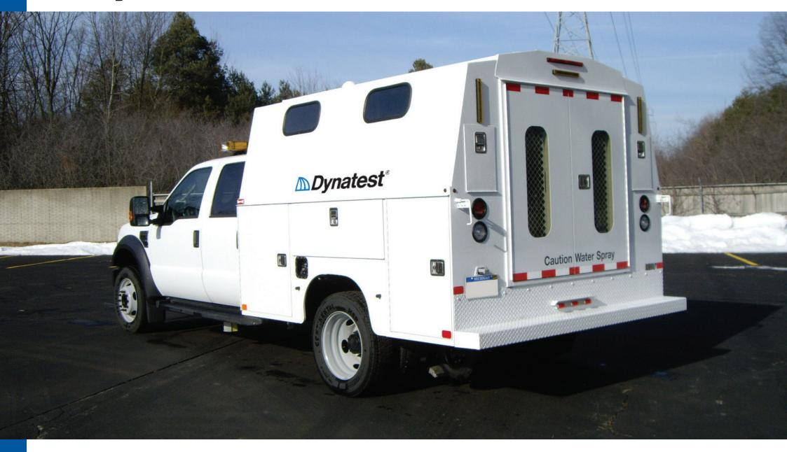
The Dynatest 6875H Highway Friction Tester is designed for maintenance testing to evaluate changes in highway pavement friction characteristics due to weathering, polishing, aging, and contaminants.
