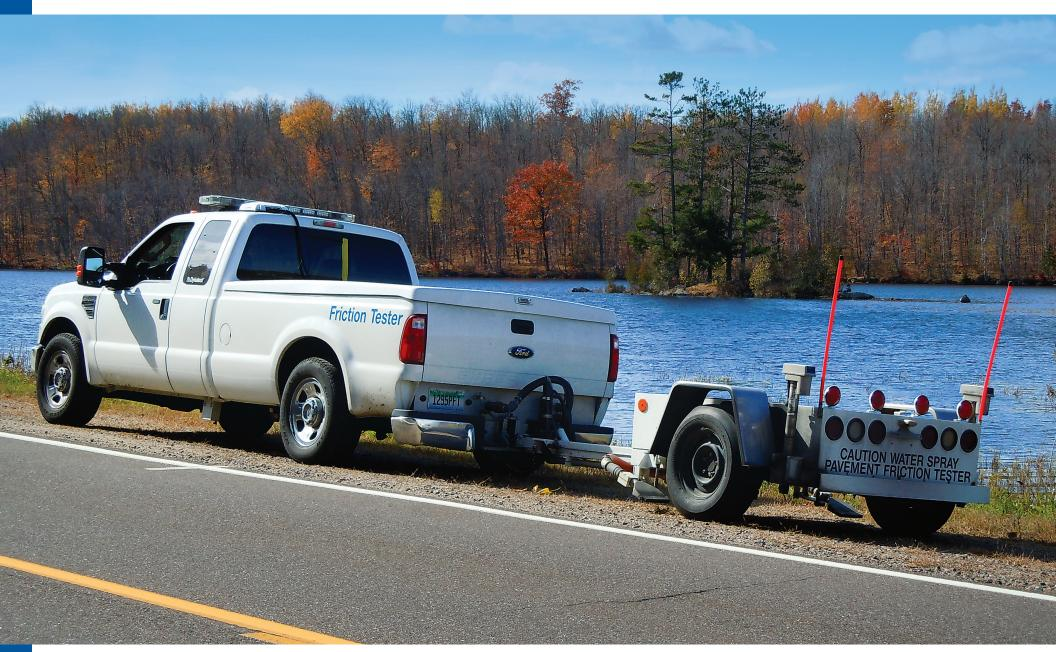
The Dynatest 1295 Pavement Friction Tester (PFT) measures the average locked wheel (skid) and peak (slip) friction characteristics on dry or self-wetted paved surfaces. It is designed for maintenance testing to evaluate the alteration of pavement friction resulting from traffic, aging and weathering.
