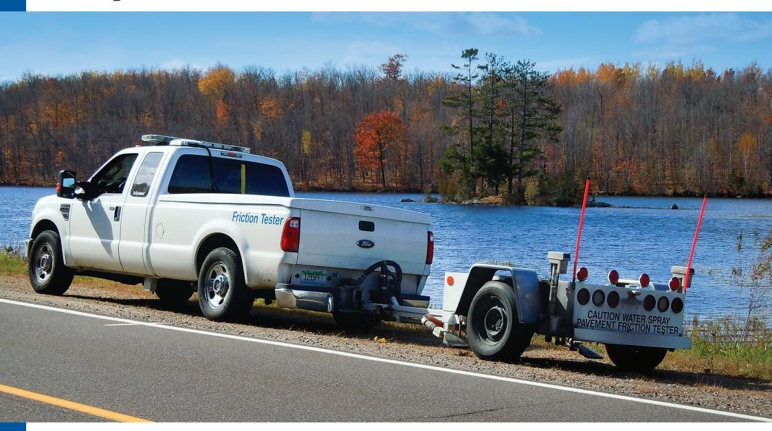
The Dynatest 1295 Pavement Friction Tester (PFT) measures the average locked wheel (skid) and peak (slip) friction characteristics on dry or self-wetted paved surfaces. It is designed for maintenance testing to evaluate the alteration of pavement friction resulting from traffic, aging and weathering.
